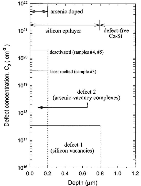
FIG. 2. Defect model used to fit the  $S$ - $z$  data. Defect 1 ( $S_{\text{trap}}=1.03$ ) accounts for vacancies within the silicon epilayer. Defect 2 ( $S_{\text{trap}}=1.00$ ) accounts for arsenic-vacancy complexes corresponding to electrical deactivation of arsenic within the highly doped region. Within the defect-free Cz-Si,  $S=1.00$ .
