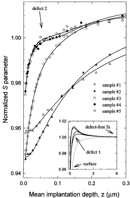
FIG. 1. Positron  $S$ - $z$  data. The  $S$  parameter values are normalized to that of bulk defect-free Cz-Si. The  $S$ - $z$  curves were obtained by solving for the diffused positron distribution and least-squares fitting to the  $S$ - $z$  data. The inset shows the  $S$ - $z$  curves extending to the maximum  $z$  measured. The  $S$ - $z$  curve for defect-free Cz-Si (dotted line) is also shown.
