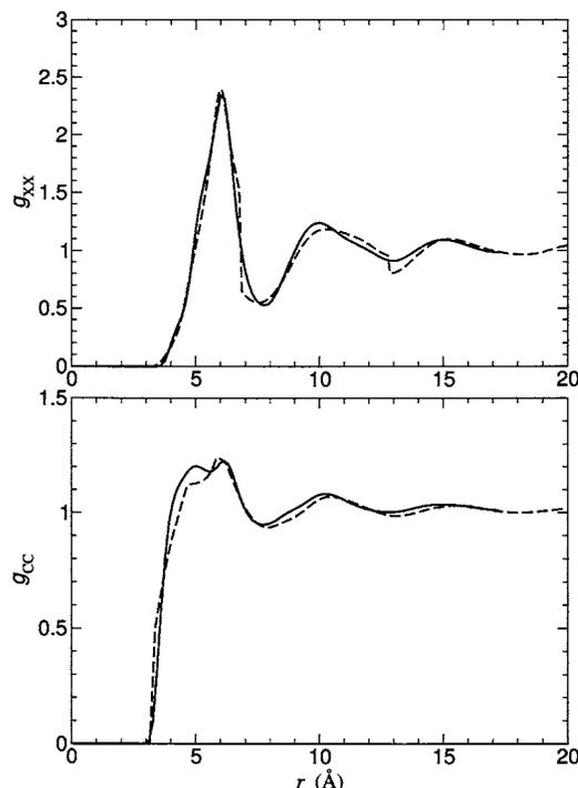
FIG. 7. From top to bottom, center-of-mass–center-of-mass ( $xx$ ) and carbon-carbon RDFs for liquid benzene. The continuous lines represent the results for SMD simulation and the dashed lines represent those for the DMD model (see Sec. III B for details).
