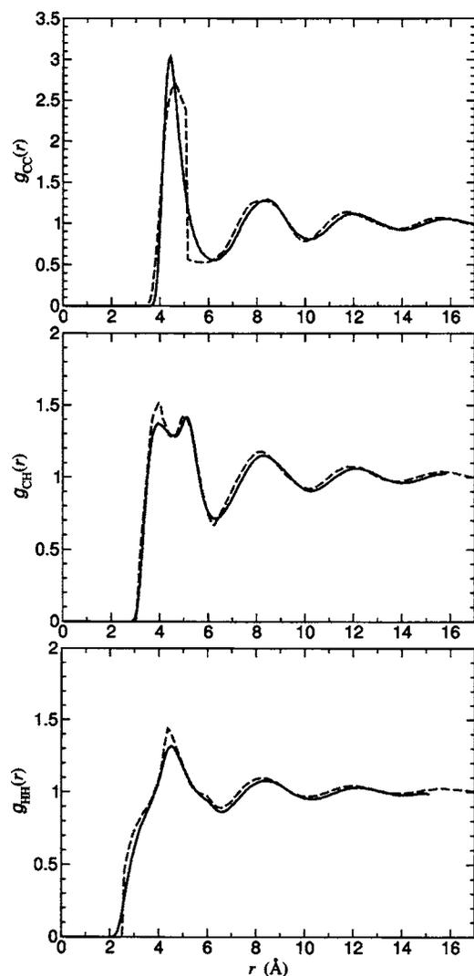
FIG. 2. From top to bottom, carbon-carbon, carbon-hydrogen, and hydrogen-hydrogen RDFs for methane at a liquidlike density of  $0.347 \text{ g/cm}^3$  and a temperature of  $126.8 \text{ K}$ . The continuous lines represent the SMD results and the dashed lines represent the DMD results. Model's parameters are given in the text.
