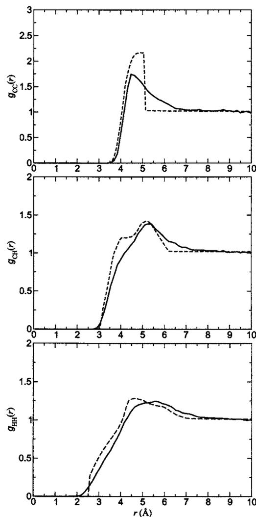
FIG. 1. From top to bottom, carbon-carbon, carbon-hydrogen, and hydrogen-hydrogen RDFs for methane at a gaseous density of  $3.47 \times 10^{-3} \text{ g/cm}^3$  and a temperature of 298 K. The continuous lines represent the SMD results and the dashed lines represent the DMD results. The parameters of the model are given in the text.
