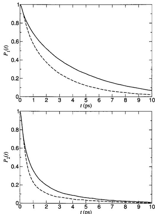
FIG. 12. Orientational time correlation functions  $P_1(t)$  and  $P_2(t)$  in liquid benzene. The continuous line corresponds to the Lennard-Jones potential and the dashed line corresponds to the DMD result.
