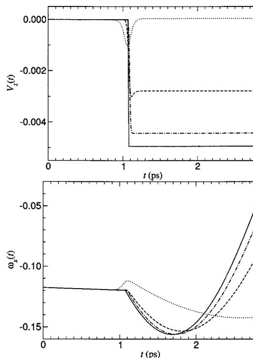
FIG. 11. Time evolution of the  $z$  component of the velocity vector (top panel) and the  $x$  component of the angular velocity vector (bottom panel) of a benzene molecule involved in a collision with another benzene molecule. The solid lines correspond to the DMD simulation. The dot, dashed, and dot-dashed lines correspond to the model interactions given by Eq. (18) with  $\alpha_2$  values of 5, 10, and 20, respectively.
